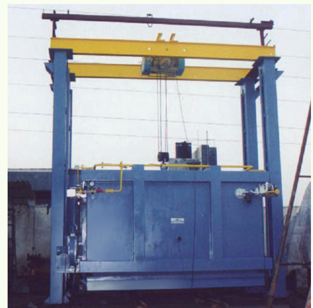
Car Bell Furnace
