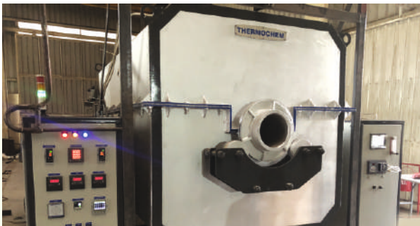
500 Kg Batch Rotary Retort Furnace
