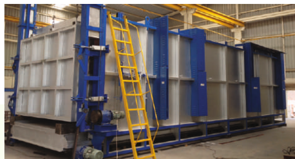
70 MT Bogie hearth Furnace - 1100 C
