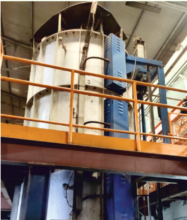
3 MT Drop Bottom Furnace - 550 C
