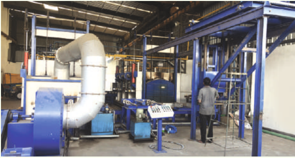
1 Ton/Hr Pusher Type NQT Furnace
