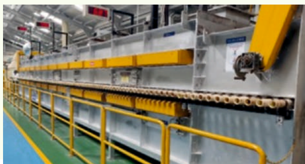
1 Ton/Hr Roller Annealing Furnace - 900 C
