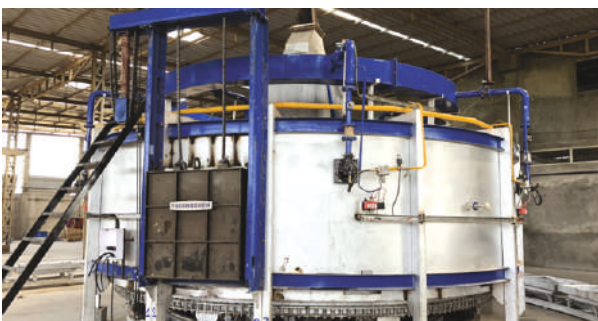
1 MT/Hr Rotary Hearth Furnace - 1200 C
